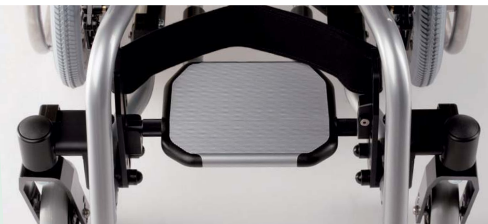
Widened front part of frame and single-panel footrest for short lower leg lengths
