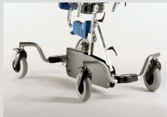
Conversion wheel kit for turning the Discovery into an Explorer
