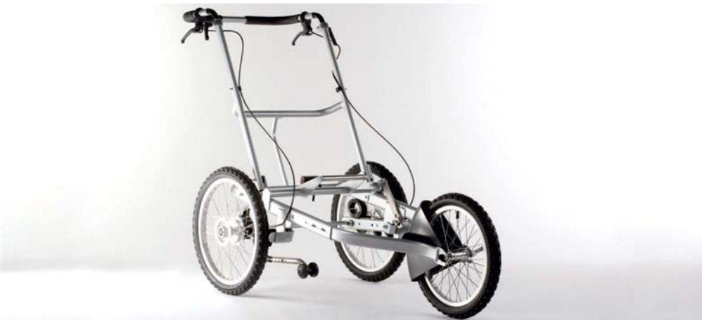
Telescoping frame with rigidly mounted front wheel
